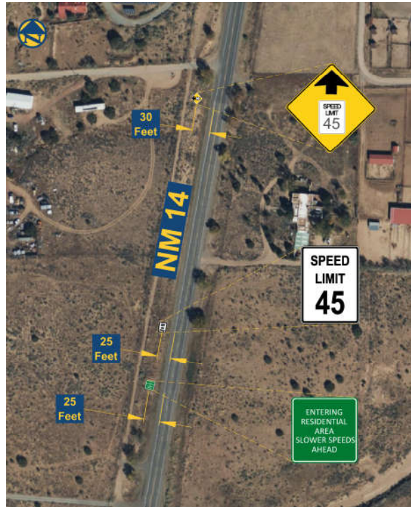
Figure 10: Existing NM 14 Southbound Approach Speed Sign Offsets
